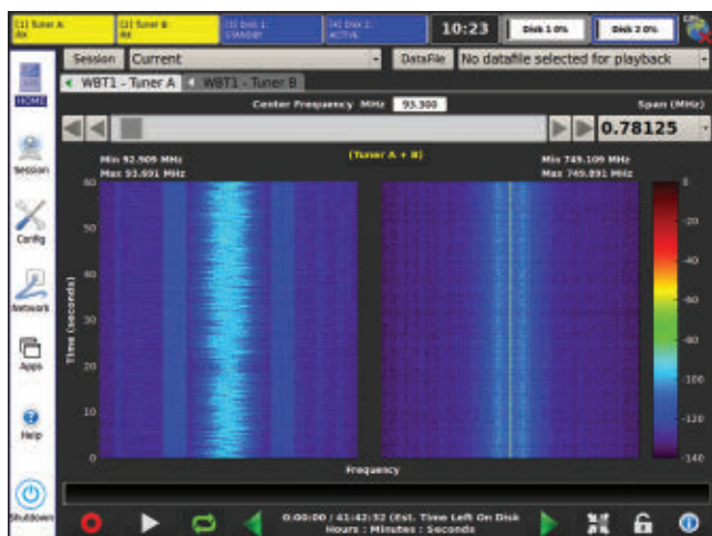
▲ Fig. 2 RF spectrogram obtained with the spectrum waterfall app.
