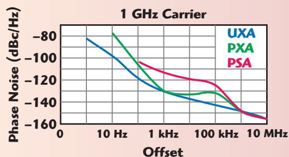
▲ Fig. 2 Compared with its high-performance predecessors — the Keysight PXA and PSA — the UXA offers improved phase noise, especially at close-in and medium offsets.
