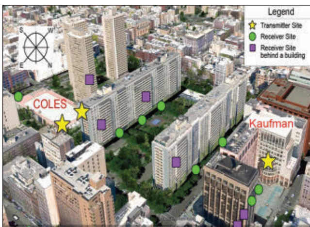
▲ Fig. 3 28 GHz measurement sites near NYU's Manhattan campus.
