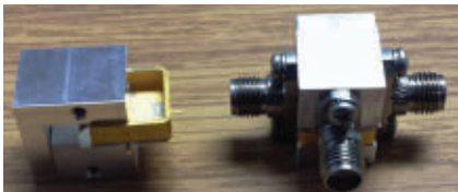
▲ Fig. 4 New test fixture for the SMT diplexer.
